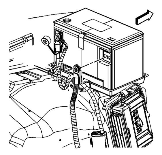
**Fig. 9: Battery Ground Negative Cable & Bolt Courtesy of GENERAL MOTORS CORP.**  1. Disconnect the negative battery cable. Refer to <u>Battery Negative Cable Disconnect/Connect Procedure</u> (Single Battery).
