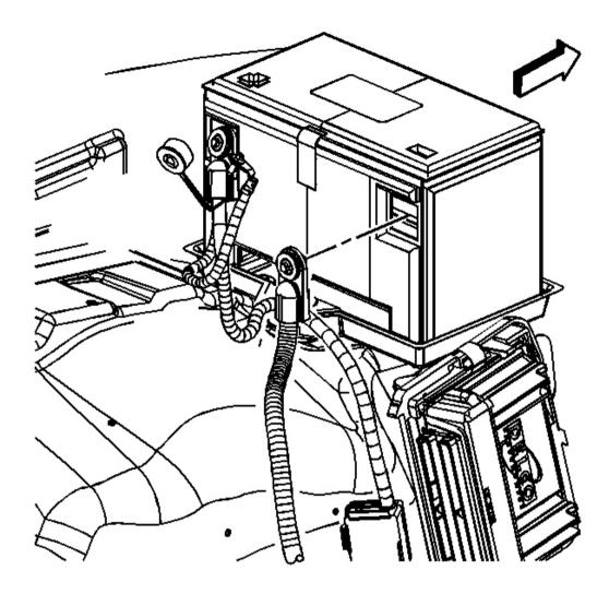
**Fig. 8: Battery Ground Negative Cable & Bolt Courtesy of GENERAL MOTORS CORP.**
