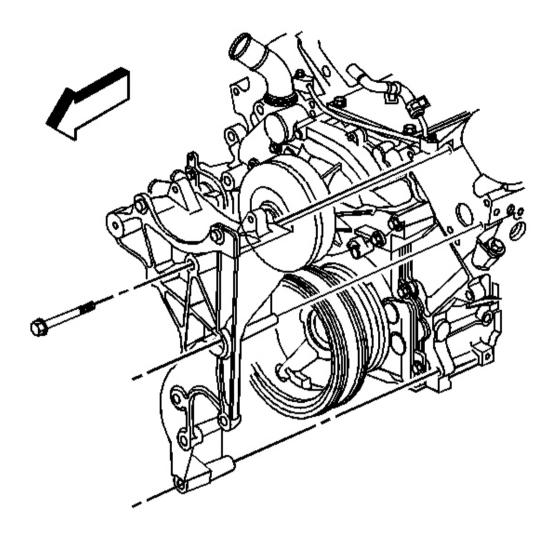
**Fig. 57: Generator Bracket** Courtesy of GENERAL MOTORS CORP.
