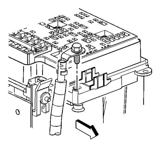
**Fig. 14: Positive Battery Cable Bolt** Courtesy of GENERAL MOTORS CORP.
