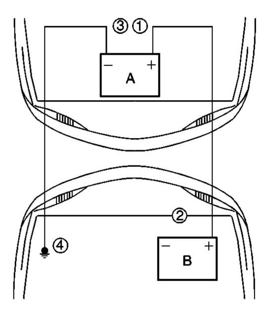
**Fig. 6: Connecting Battery Terminal Jumpers Courtesy of GENERAL MOTORS CORP.**
