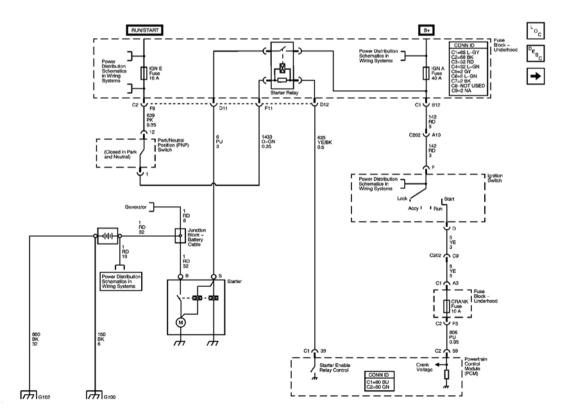
**Fig. 1: Starting Schematics** Courtesy of GENERAL MOTORS CORP.
