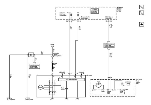
**<u>Fig. 2: Charging Schematics</u> Courtesy of GENERAL MOTORS CORP.**
