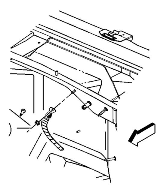
**Fig. 37: Ground Strap Nut** Courtesy of GENERAL MOTORS CORP.
