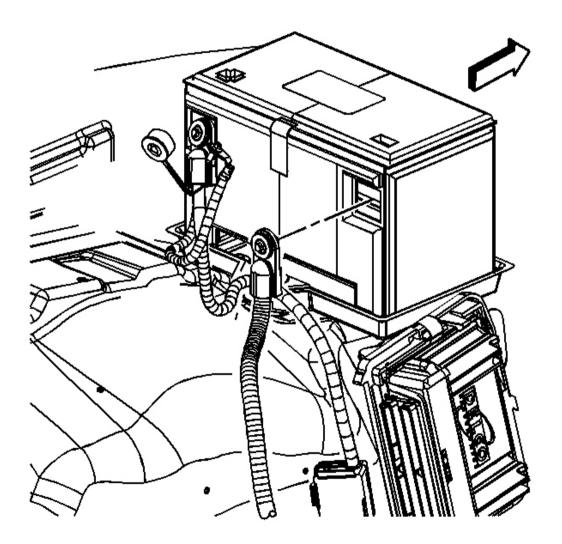
**Fig. 13: Battery Ground Negative Cable & Bolt** Courtesy of GENERAL MOTORS CORP.
