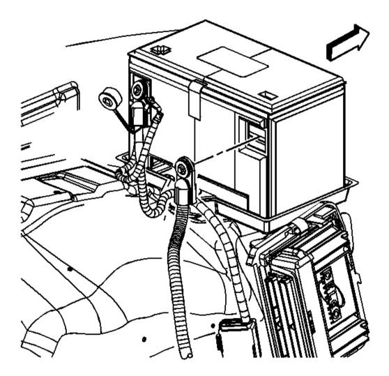
Fig. 23: Battery Ground Negative Cable & Bolt Courtesy of GENERAL MOTORS CORP.
