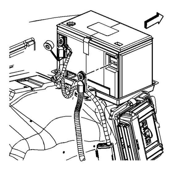
**Fig. 32: Battery Ground Negative Cable & Bolt** Courtesy of GENERAL MOTORS CORP. 5. Connect the negative battery cable. Refer to <u>Battery Negative Cable Disconnect/Connect Procedure</u> (Single Battery).
