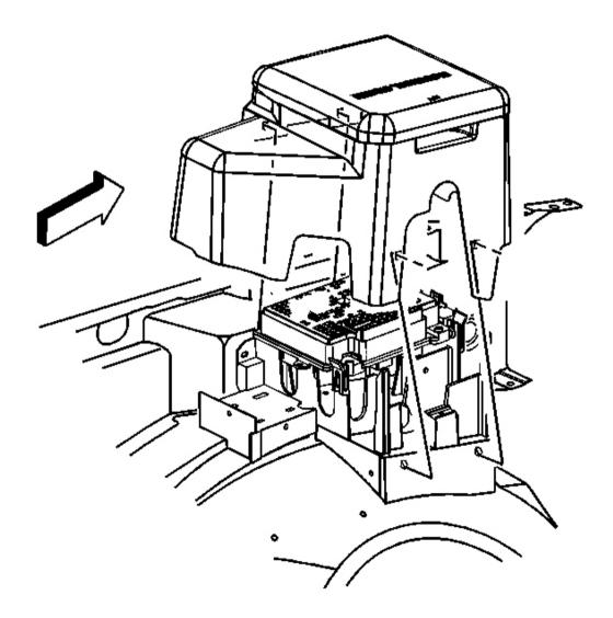
**Fig. 40: Starter Motor Relay** Courtesy of GENERAL MOTORS CORP.
